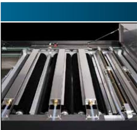
Round brushes technology for top quality plates. IN-LINE & ALL-IN-ONE machine. First in this format.
